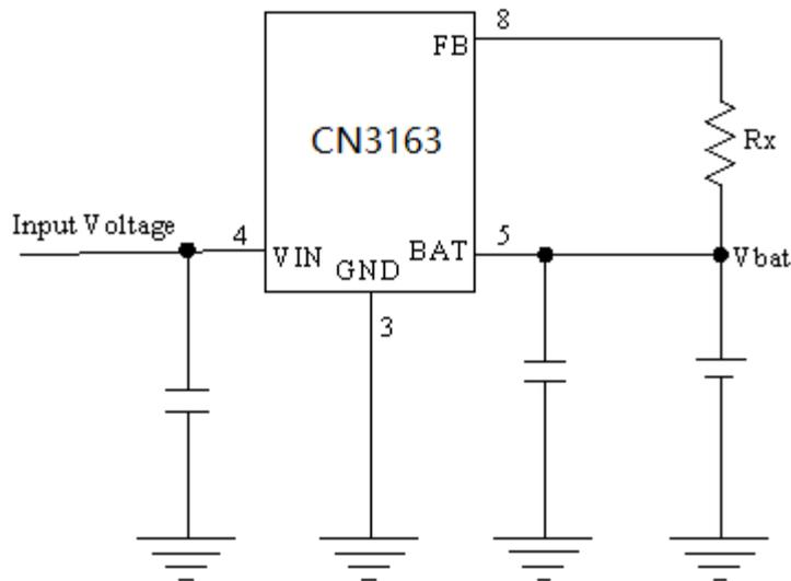
**Figure 5 Adjusting Regulation Voltage in Constant Voltage Mode**
