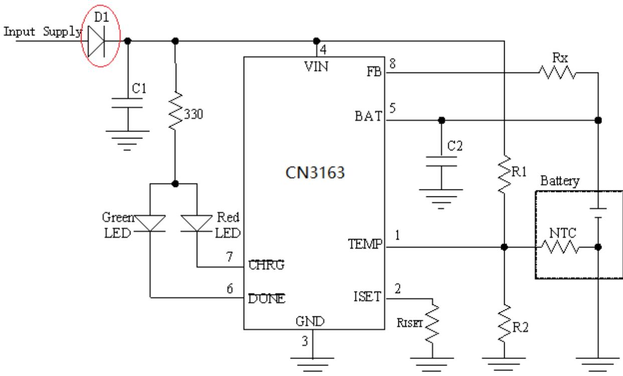
Figure 6 Adding Diode D1 to Suppress Voltage Spike
