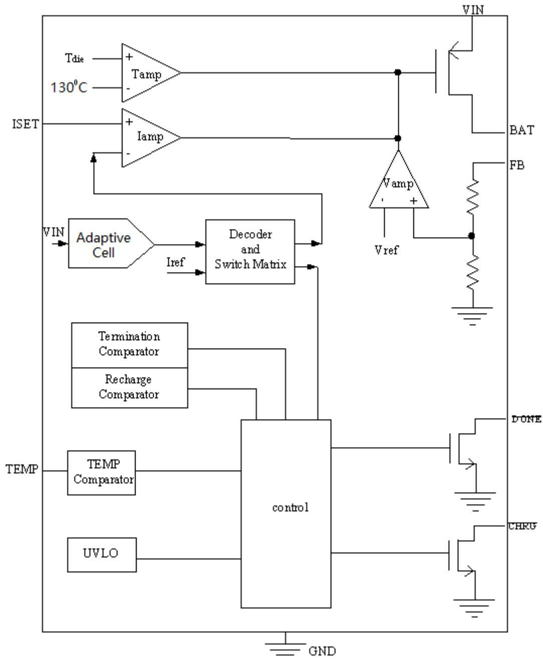
Figure 3 Block Diagram
