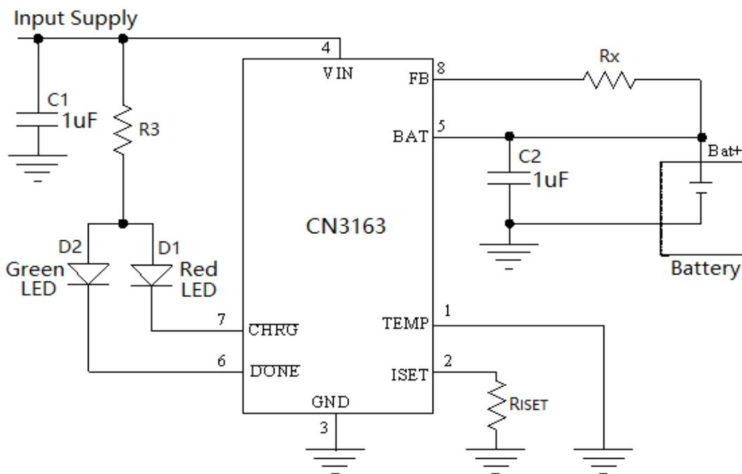
Figure 2 Application Circuit(Adjust Constant Voltage Level with Rx)
